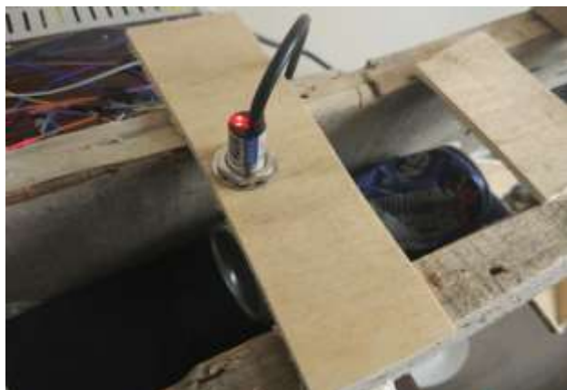
Fig. 4. Response of inductive sensor to metal material
