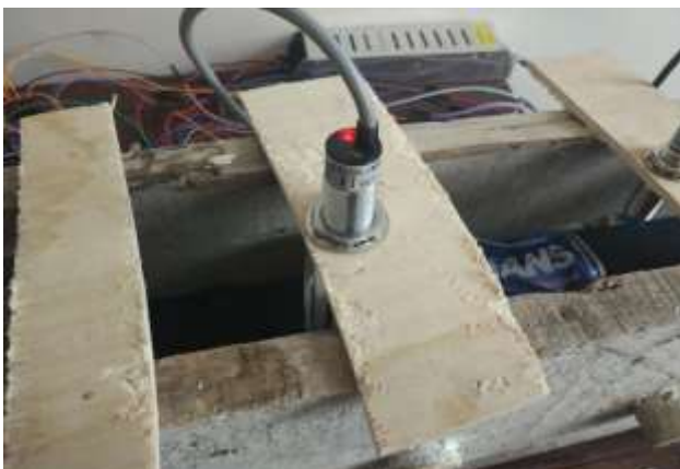
Fig. 3. Response of capacitive sensor to metal material
