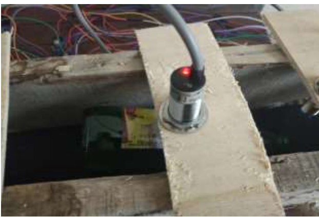
Fig. 1. Response of capacitive sensor to glass material
