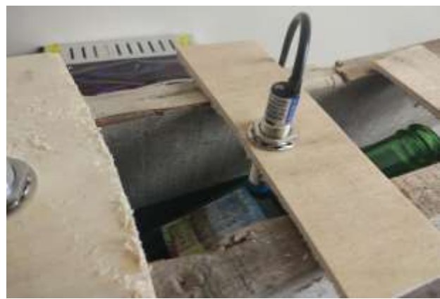
Fig. 2. Response of inductive sensor to glass material
