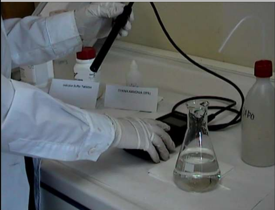
Figure 1: The conductivity meter was used for the measurement of the specific conductivity.
