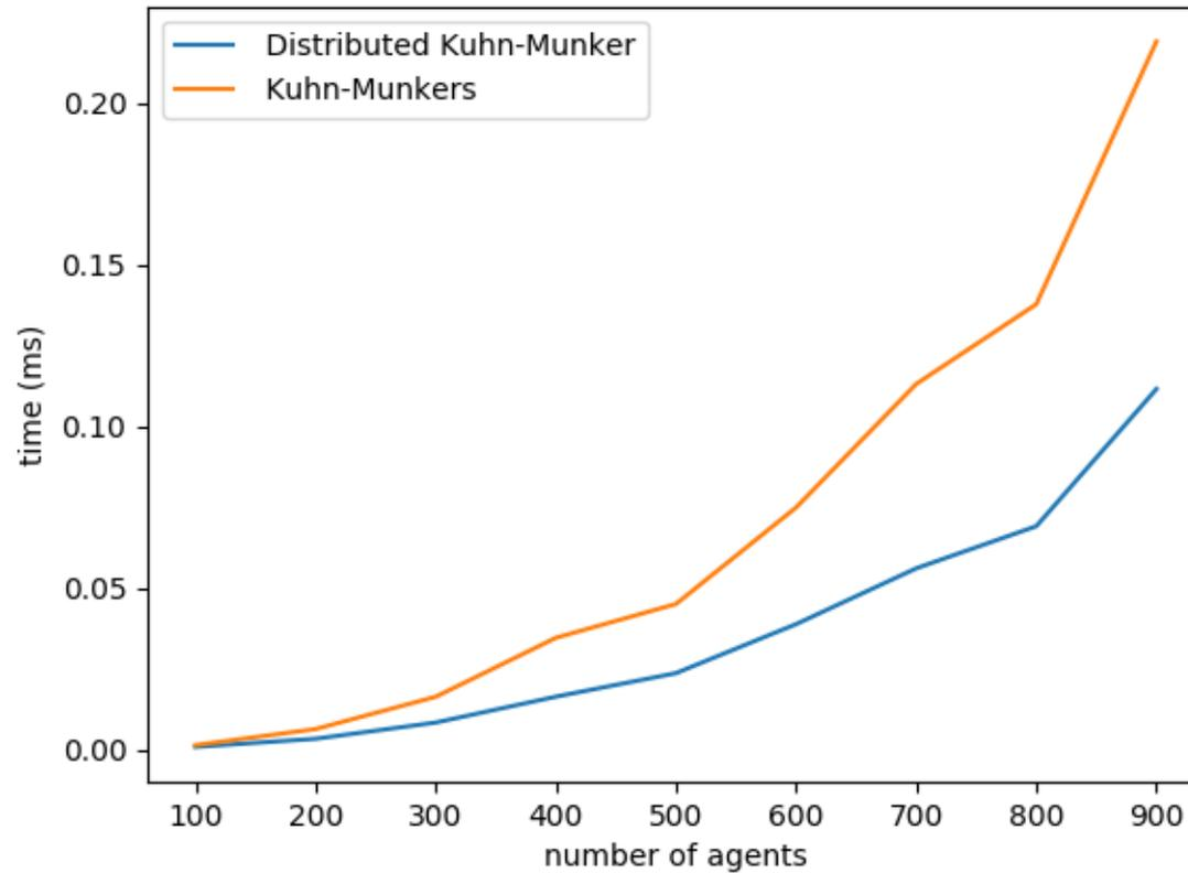
Comparison of Distributed Kuhn-Munkers and Kuhn-Munkers algorithms for range of number of agents from 100 to 1000
