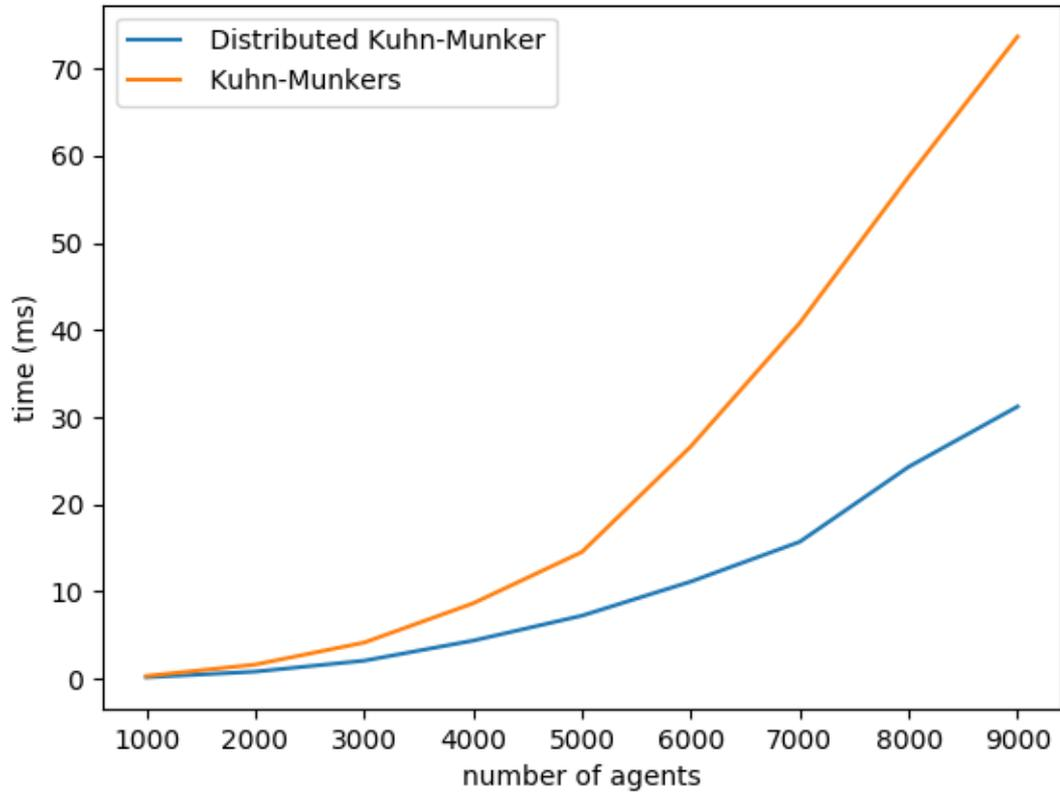
Comparison of Distributed Kuhn-Munkers and Kuhn-Munkers algorithms for range of number of agents from 1000 to 9000
