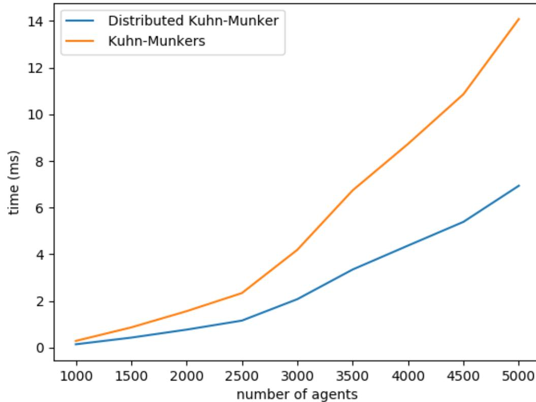
Comparison of Distributed Kuhn-Munkers and Kuhn-Munkers algorithms for range of number of agents from 1000 to 5000
