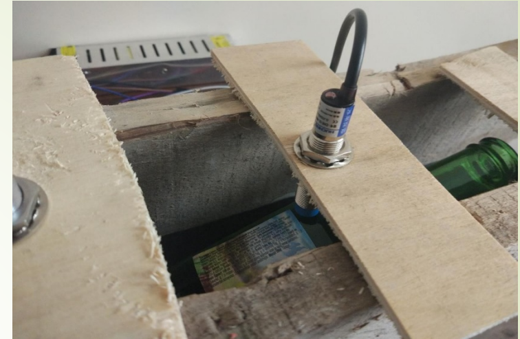
Fig. 2. Response of inductive sensor to glass material
