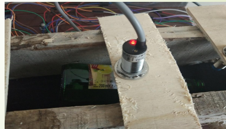
Fig. 1. Response of capacitive sensor to glass material
