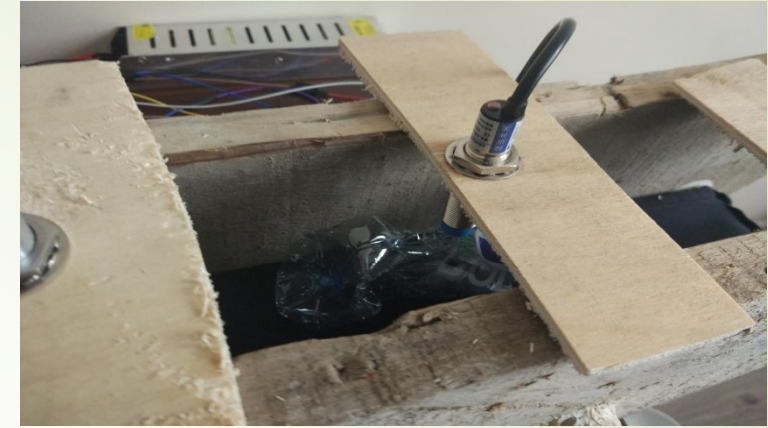
Fig. 6. Response of inductive sensor to plastic material
